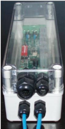
SLAMMO V5 - in IP54 and IP67 versions - is supplied with four off M20 glands that are suitable for cables with an OD of 6 to 12mm. If the cable diameter (eg for DMX) is smaller, insert the separate reducing seal which will change the gland to suiting 5 to 9mm OD cables. Also supplied with the IP54 version is an M20 blind screw for applications where only 3 of the 4 possible glands are needed.
